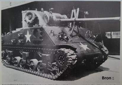
Newly modified at the Tokyo Ordnance Center in September 1950 this Sherman M4A3 was one of many which had its 75-mm M3 gun replaced by a 76-mm gun for use in Korea. The original turret was retained and the recoil guard of the 76 was modified to let it fit in.
