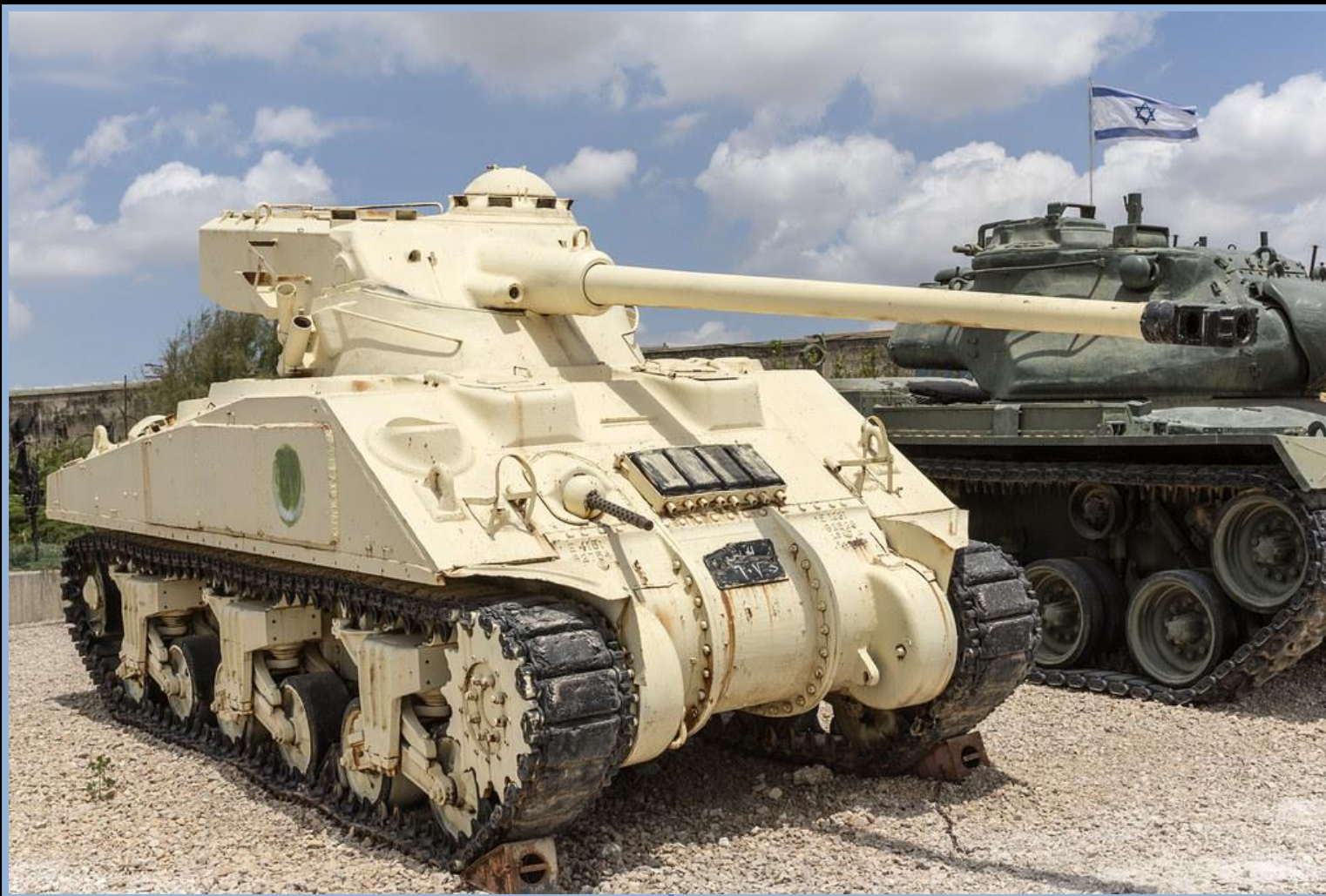
Sherman M4A4 hull Retrofitted with an M4A2 engine + FL 10 Turret
